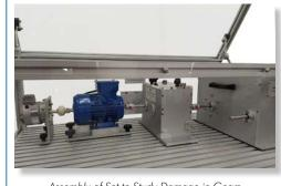
Assembly of Set to Study Damage in Gears "MDU-SSDG" in the MDU Base Unit, "MDU-UB" with the Break and Load Unit "MDU-BLU"
