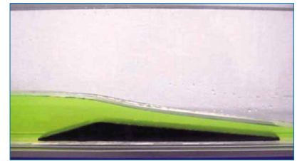
CFVC. Crump weir
