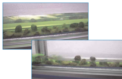
CFPLR. Artificial roughened bed (3 different models)
