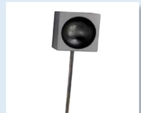
TA9/300. Drag Model of Hemisphere Concave to Airflow
