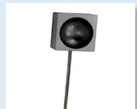
TA9/300. Drag Model of Hemisphere Concave to Airflow
