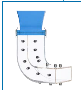
ATB/PDB. Pressure Distribution in a Pipe Bend
