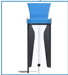
ATB/BL. Model to Study the Boundary Layer
