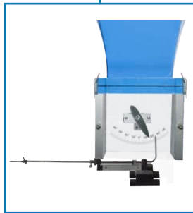
ATB/DF. Model to Study the Drag Forces
