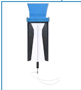
ATB/BP. Model to Study Bernoulli's Principle
