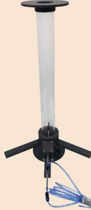
HVCC-CTPP. 64 mm. diameter duct and pressure taking with Pitot
