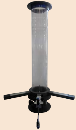
HVCC-CTPG. 114 mm. diameter duct and pressure taking with Pitot
