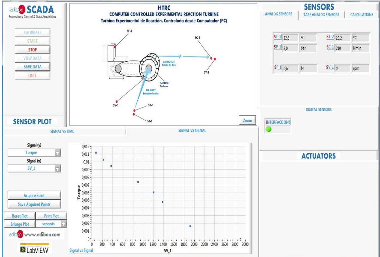
Signal versus signal chart where any of the measured or calculated variables can be represented. Mechanical power vs turbine speed.
