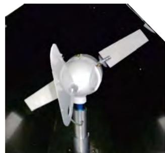
Aerogenerator with two blades
