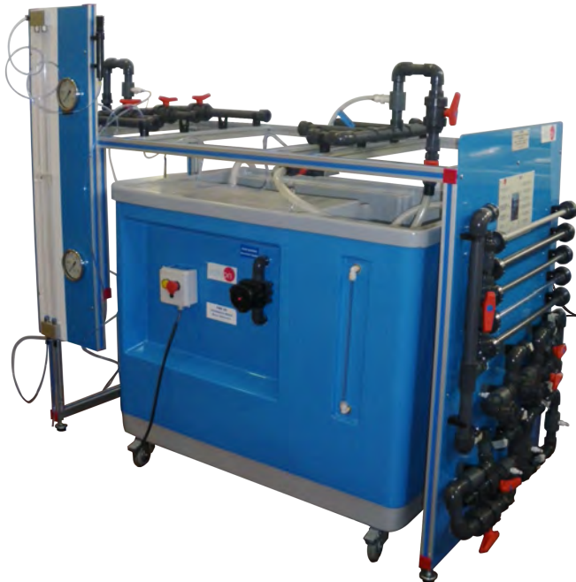
① Unit: AMTC. Computer Controlled Pipe Network Unit, with Hydraulics Bench (FME00)
