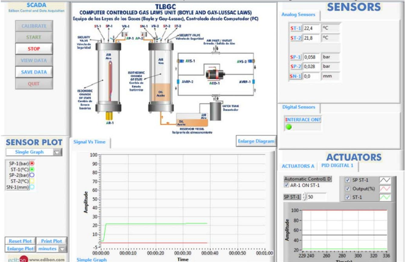
This screen shows how the increase of the temperature inside the vessel for the investigation of isochoric change of state implies an increase of the pressure.
