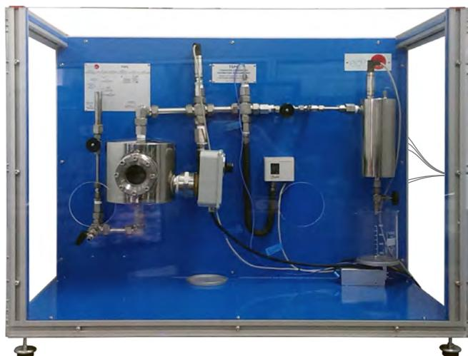
① Unit: TSPC. Computer Controlled Saturation Pressure Unit
