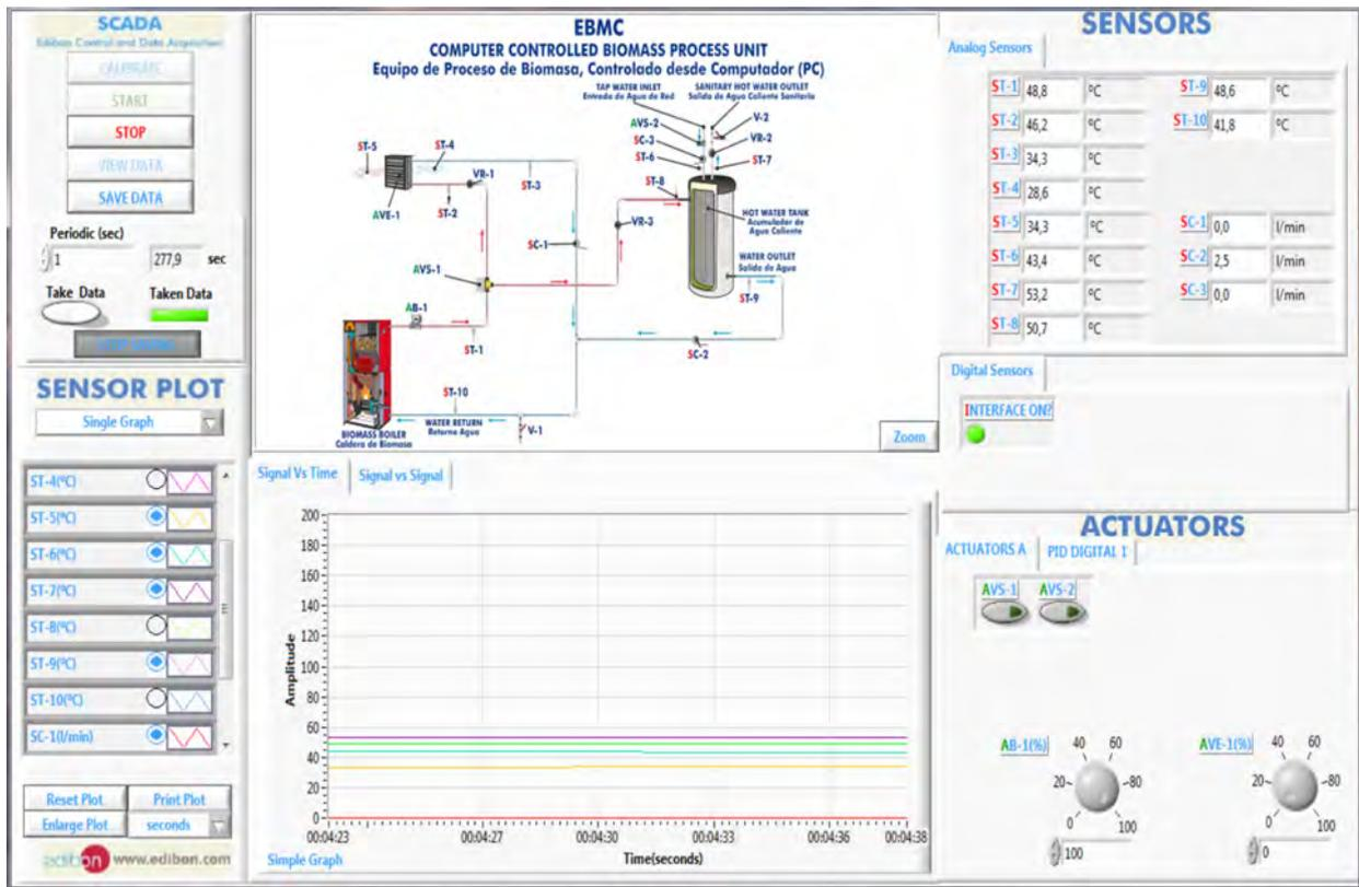
When the solenoid valve (AVS-1) is activated, the heating water can go towards both primary circuits and the flow can be regulated from 0 to 100% (AB-1 pump).
