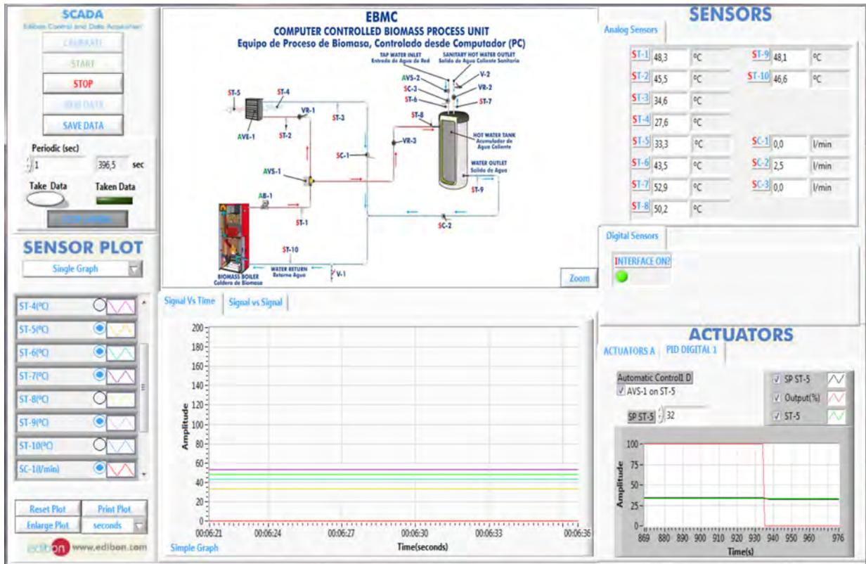
The software enables to plot the signal of one sensor versus the signal of another sensor.
