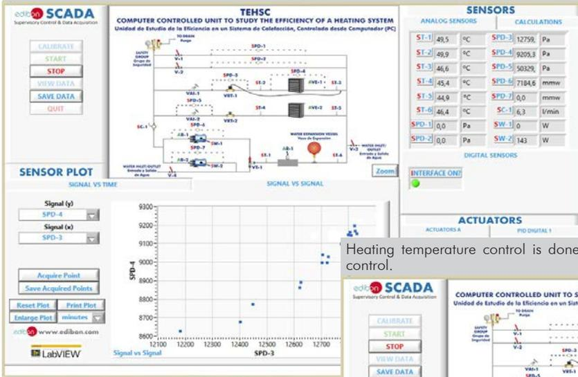
Heating temperature control is done through a PID control and a two point temperature control.
