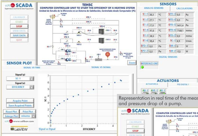
Representation in real time of the measured and calculated magnitudes. Charts for temperature and pressure drop of a pump.
