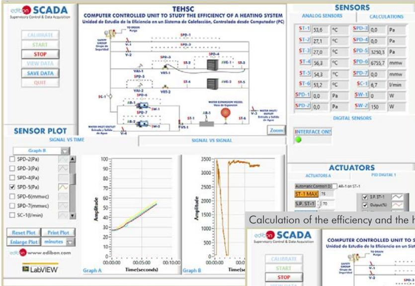
Calculation of the efficiency and the hydraulic power.
