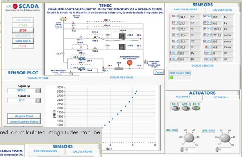
Signal versus signal chart where any of the measured or calculated magnitudes can be represented. Flow versus efficiency.
