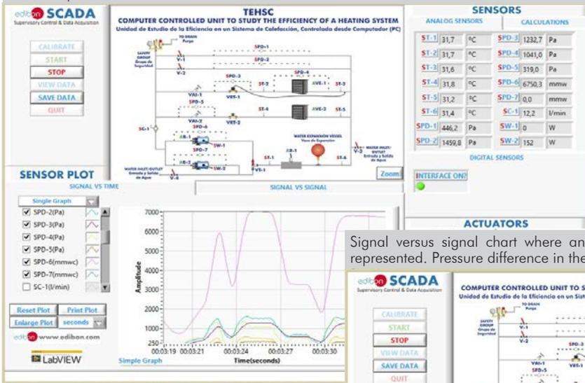
Signal versus signal chart where any of the measured or calculated magnitudes can be represented. Pressure difference in the angle seat valve versus flow.
