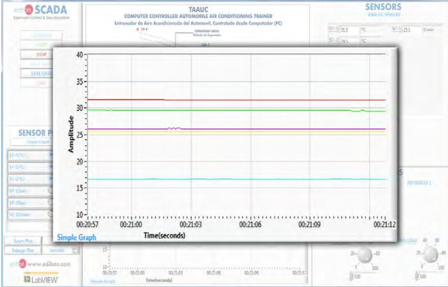
PID control of the compressor. When the set point is reached at the temperature sensor (ST-5), the compressor is turned off.
