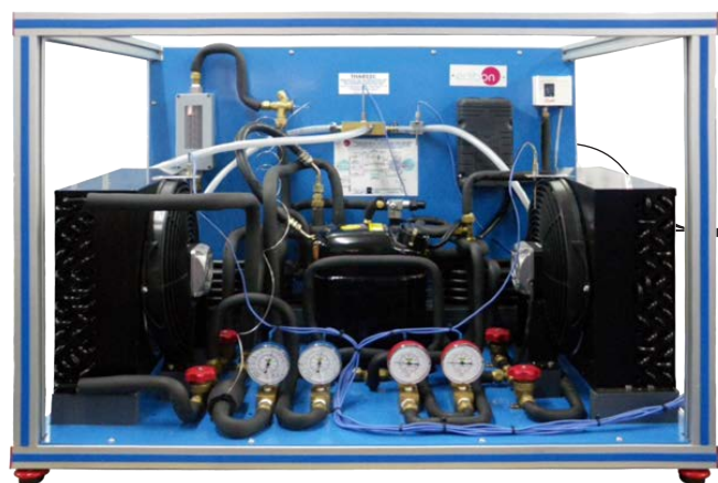
① Unit: THAR22C. Computer Controlled Heat Pump, Refrigeration and Air Conditioning Unit (two condensers (water and air) and two evaporators (water and air))
