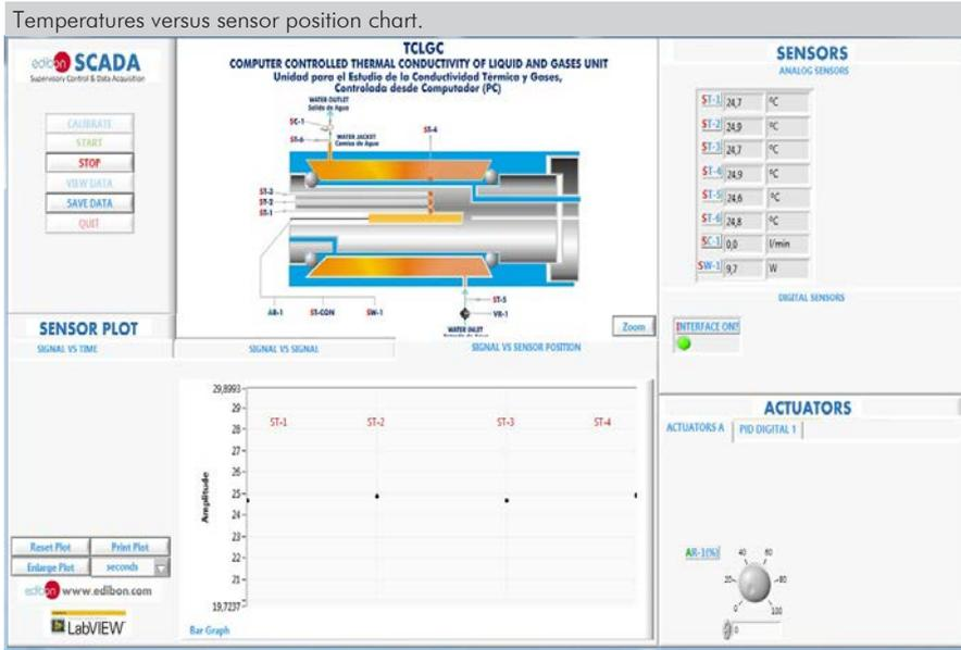
Representation in real time of the measured magnitudes. Heating temperature control is done through a PID control.
