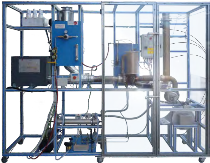
① Unit: TGDEPC. Two-Shaft Gas Turbine/Jet Engine
