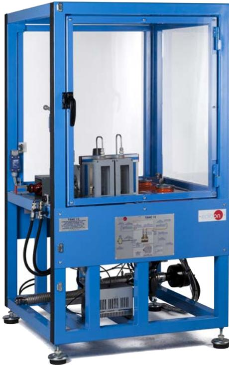
① Unit: TBMC12. Computer Controlled Test Bench for Single-Cylinder and Two-Cylinders Engines, 11 kW
