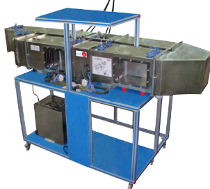
TRAMC/4. Complete Air Conditioning System Model (+)
