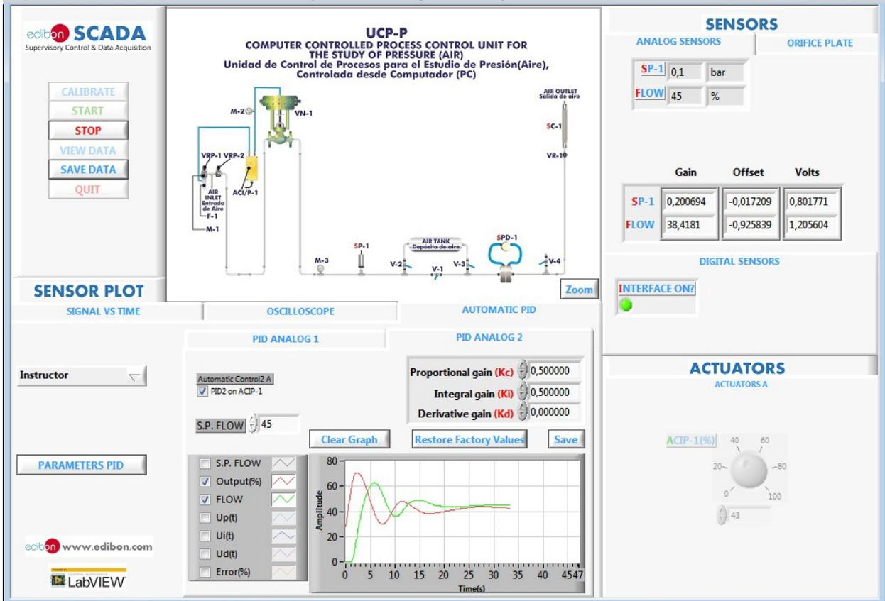
Representation in real time of the measured magnitudes. Pressure response when a change is introduced in the signal of the control valve.
