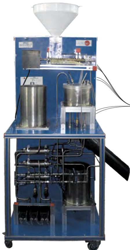
① Unit: UESLC. Computer Controlled Solid-Liquid Extraction Unit
