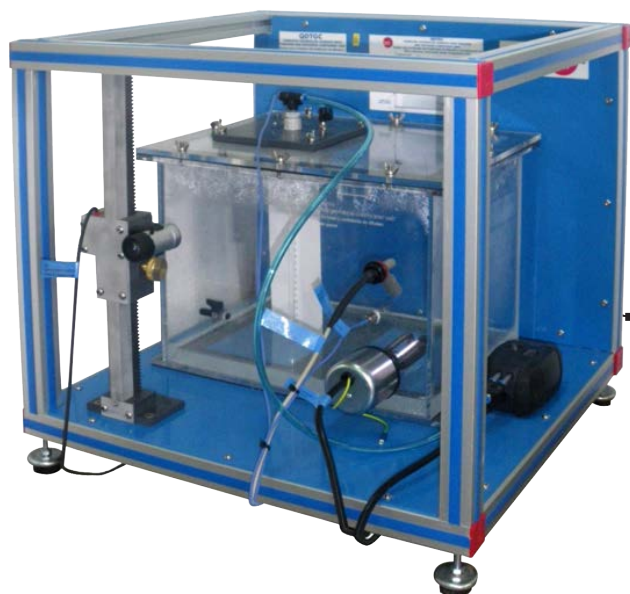
① Unit: QDTGC. Computer Controlled Gaseous Mass Transfer and Diffusion Coefficient Unit
