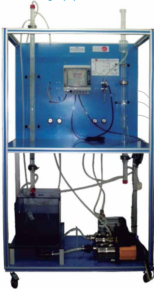
① Unit: CAPC. Wetted Wall Gas Absorption Column
