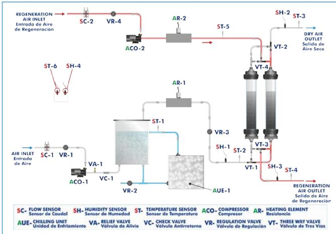
① Unit: QSAC. Computer Controlled Adsorptive Air Drying Unit
