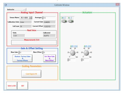
The teacher and the students can calibrate the unit with a password provided by EDIBON. The teacher can restore the factory calibration any time.
