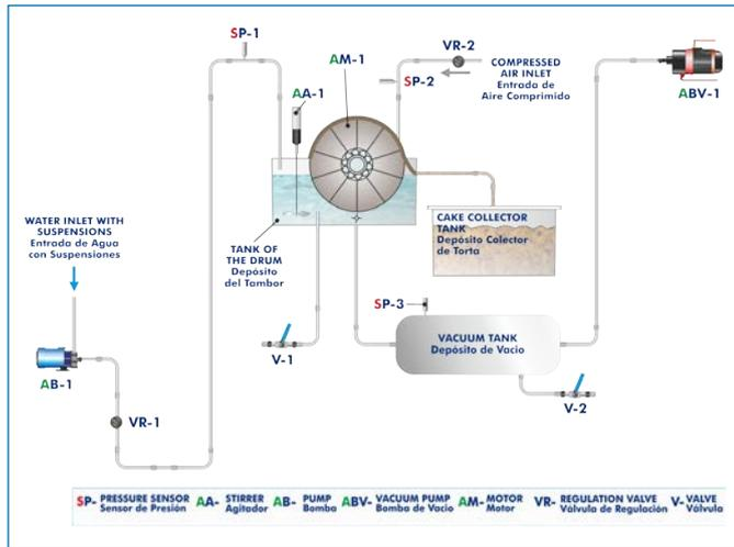
① Unit: PFTC. Computer Controlled Drum Cell Filter
