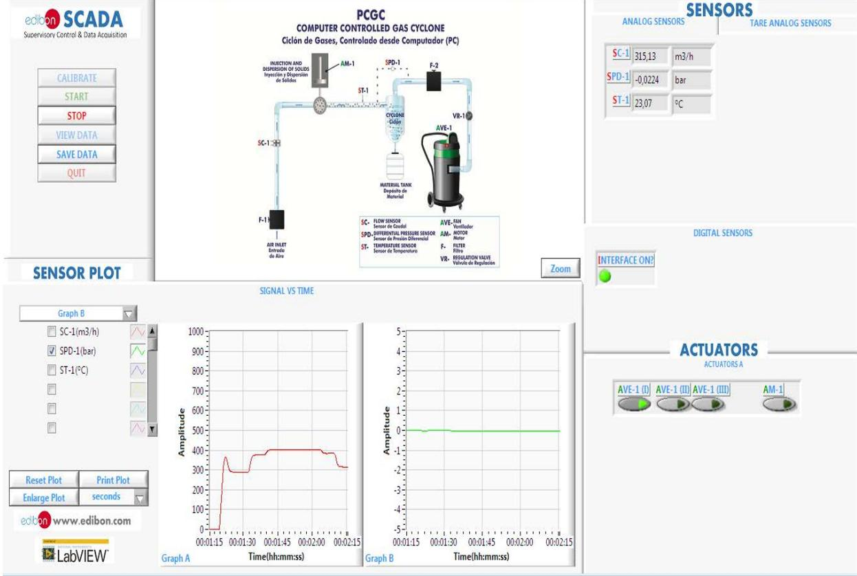
Representation in real time of the measured magnitudes. Representation of air flow and temperature and pressure drop in the cyclone.
