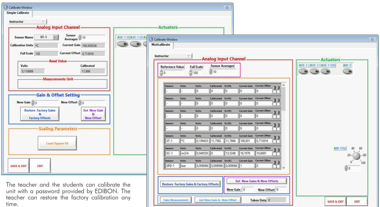
The teacher and the students can calibrate the unit with a password provided by EDIBON. The teacher can restore the factory calibration any time.
