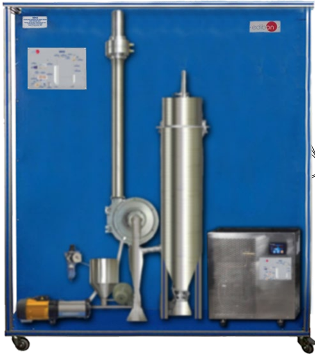
① Unit: SDCC. Computer Controlled Spray Dryer and Chiller Unit
