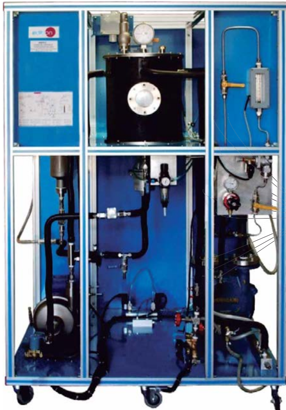
① Unit: AEHC. Hydrogenation Unit
