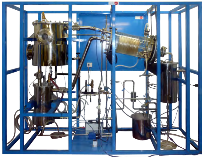
① Unit: QEDC. Computer Controlled Batch Solvent Extraction and Desolventising Unit
