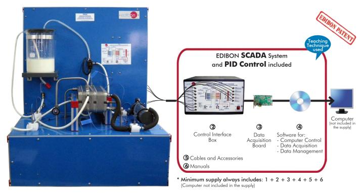
1 Unit: PASC. Computer Controlled Laboratory Pasteurizer
