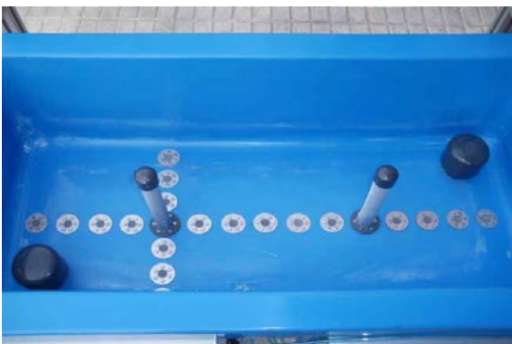
Detail of tank inside (pressure tappings, wells, etc)
