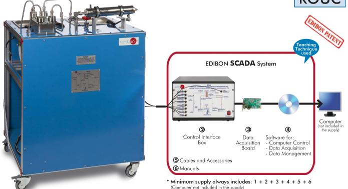
① Unit: ROUC. Computer Controlled Reverse Osmosis/ Ultrafiltration Unit
