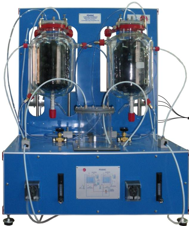
① Unit: PDANC. Computer Controlled Anaerobic Digester
