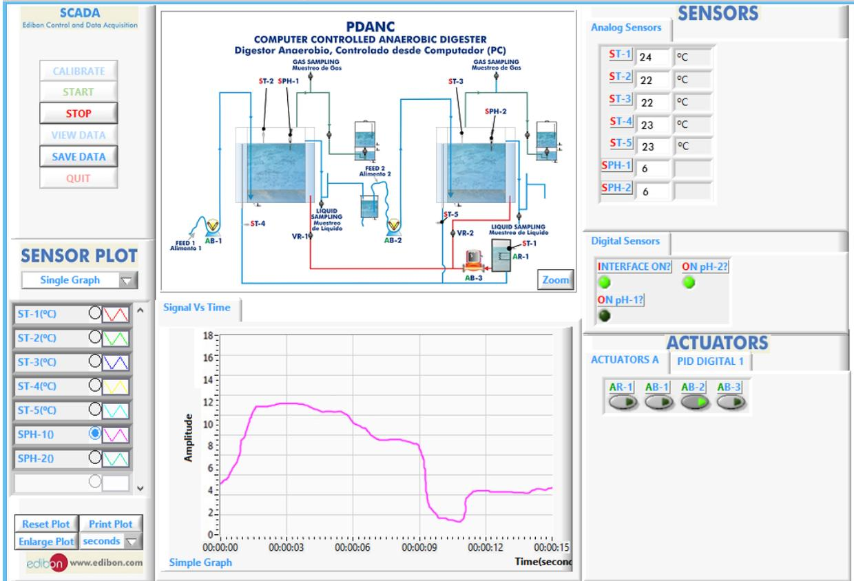
Representation in real time of the measured magnitudes. Variation of the digester temperatures versus time.
