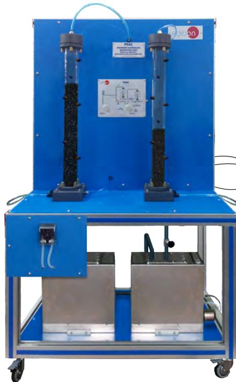
① Unit: PEAC. Computer Controlled Adsorption Unit
