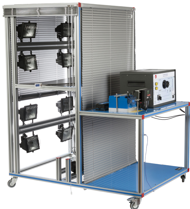
① Unit: EESFC. Computer Controlled Photovoltaic Solar Energy Unit
