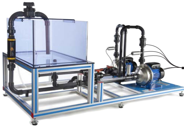
① Unit: PBSPC. Computer Controlled Series/Parallel Pumps Bench
