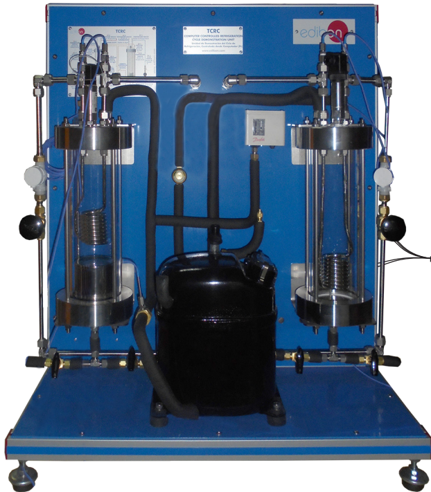
① Unit: TCRC. Computer Controlled Refrigeration Cycle Demonstration Unit
