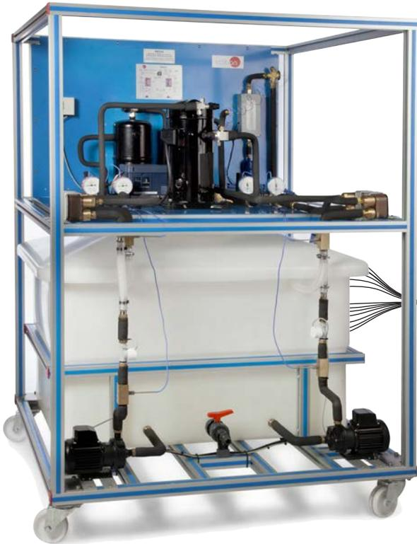
① Unit: TRCVC. Computer Controlled Vapour-Compression Refrigeration Unit
