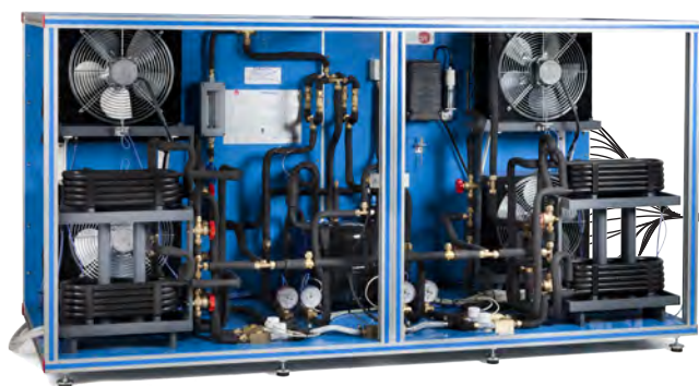
① Unit: THIBAR44C. Computer Controlled Reversible Heat Pump + Air Conditioning + Refrigeration with 4 Condensers and 4 Evaporators (Water/Air)
