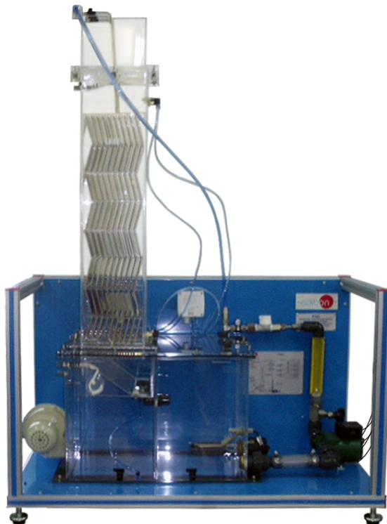
① Unit: TTEC. Computer Controlled Bench Top Cooling Tower
