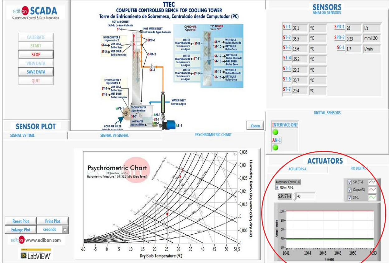
Signal versus signal chart where any of the measured variables can be represented.
