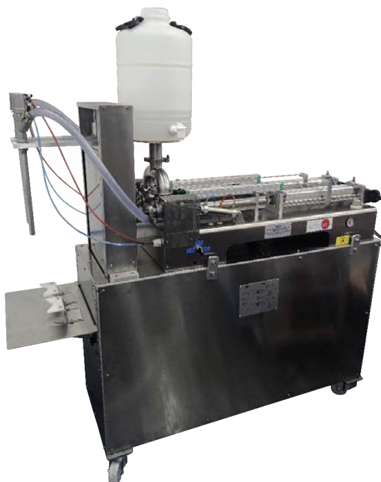
① Unit: EDLC. Computer Controlled Liquid Packaging Teaching Unit
