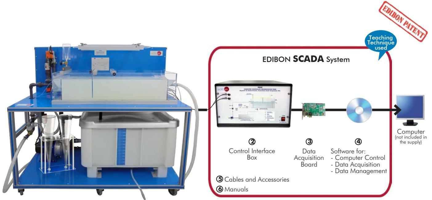
① Unit: PDSC. Computer Controlled Sedimentation Tank
