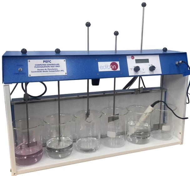
① Unit: PEFC. Computer Controlled Flocculation Test Unit
