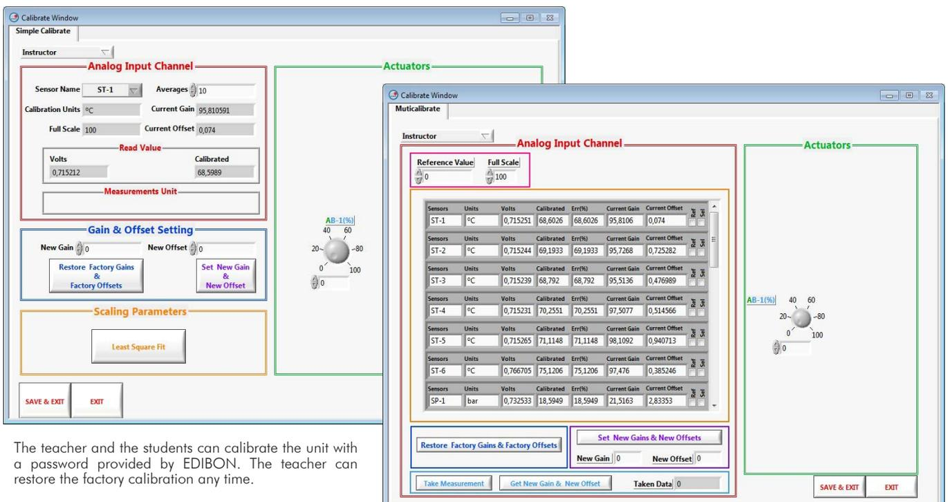
The teacher and the students can calibrate the unit with a password provided by EDIBON. The teacher can restore the factory calibration any time.
