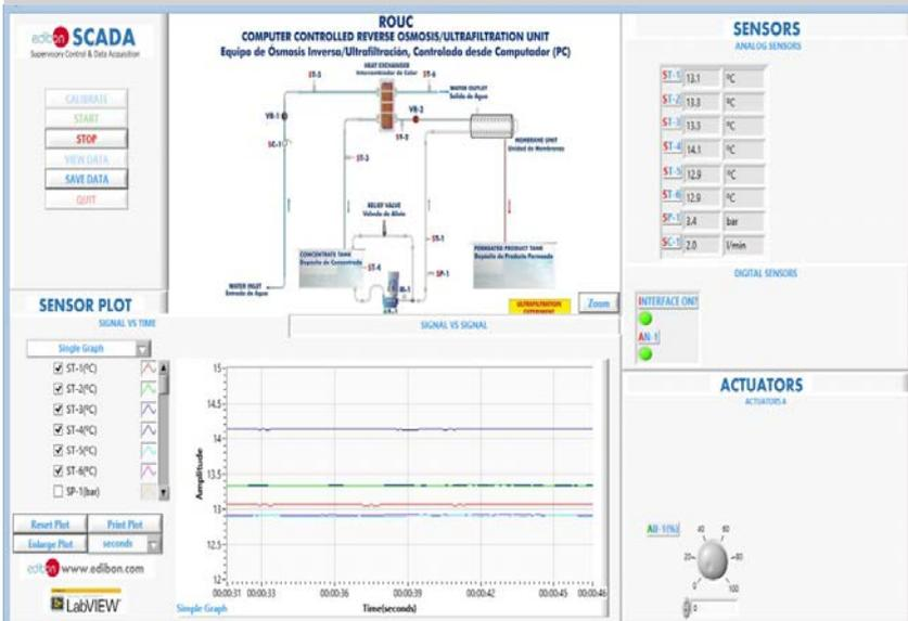
Representation in real time of the measured magnitudes. Chart with pressure measurement evolution.
