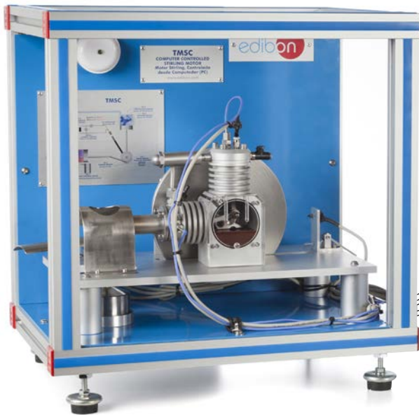
① Unit: TMSC. Computer Controlled Stirling Motor
