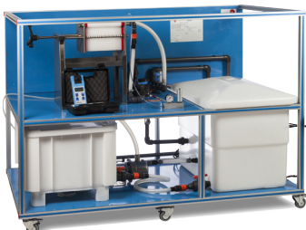
① Unit: AFPMC. Computer Controlled Plate and Frame Filter Press
