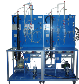
① Unit: EDPAC. Computer Controlled Double Effect Rising Film Evaporator
